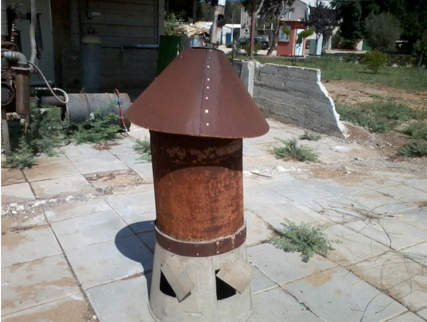
Figure 2. Udine pyrolysis system modified in the Volcani Center to treat agricultural wastes
