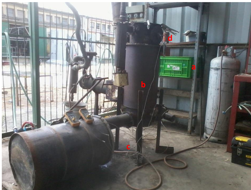
Figure 1. BEK, PowerLabs pyrolysis system modified in the Volcani Center for agricultural wastes
